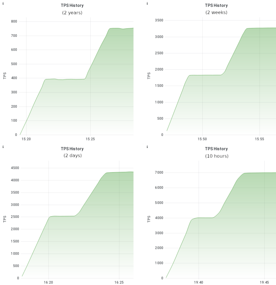
Figure 6.3.: TPS (withdrawals and payments per second) shown with different values for LOOKAHEAD_SIGN. In each experiment we started two times 600 wallets, and we can see clearly how much their speed improved.
