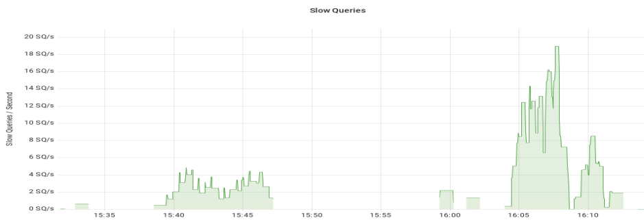
Figure A.15.: Number of slow queries per second, calculated from the database's logs, which are preprocessed by Promtail. It is taken from log_min_duration_statement based on the filter duration: so make sure the setting is enabled.
